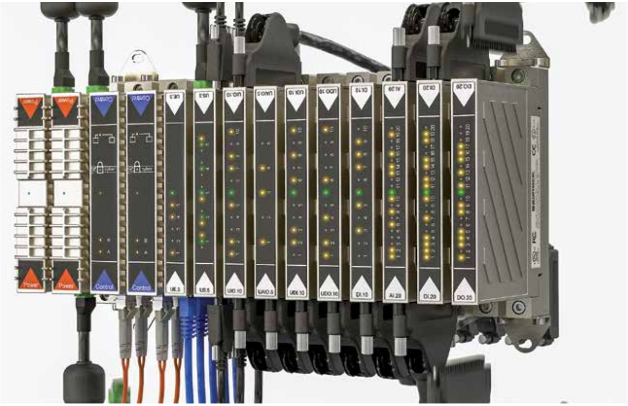
FIG. 1. Each module of this Bedrock Open Secure Automation system has its full cryptographic identity, which prevents it from being cloned or counterfeited.
