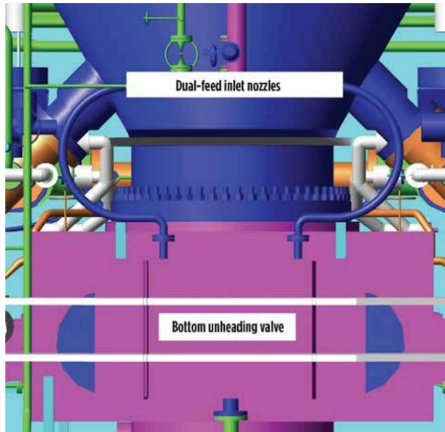
FIG. 2. Dual-inlet elevation plan.
