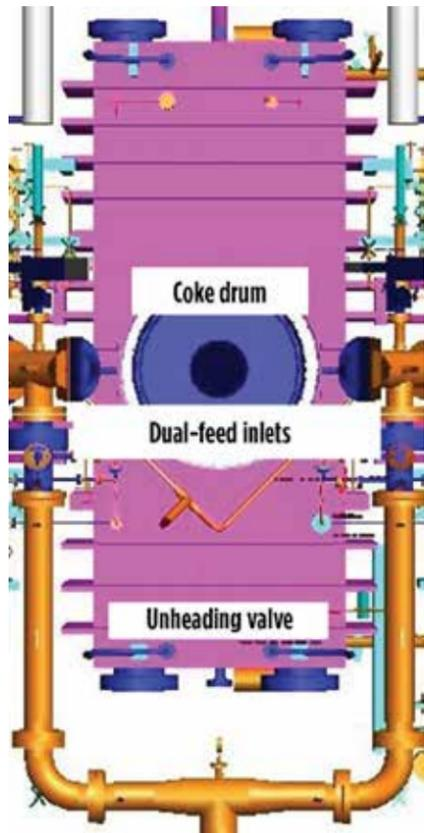
FIG. 1. General arrangement of the BHTS dual-inlet technology.
