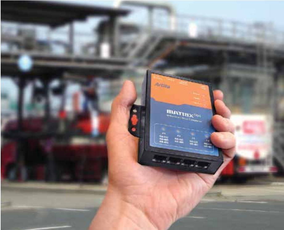
FIG. 1. The TCP-X-Unit, a suite comprising the Matrix-504 microcomputer and suitable software, translates RS-232-signals from older field devices for the modern terminal management system OpenTAS.
